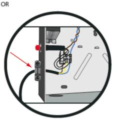
• Through the optional AC input receptacle. **Note:** the brown and blue wires must be twisted together from the point of entry at the AC input receptacle to the Terminal Block.
